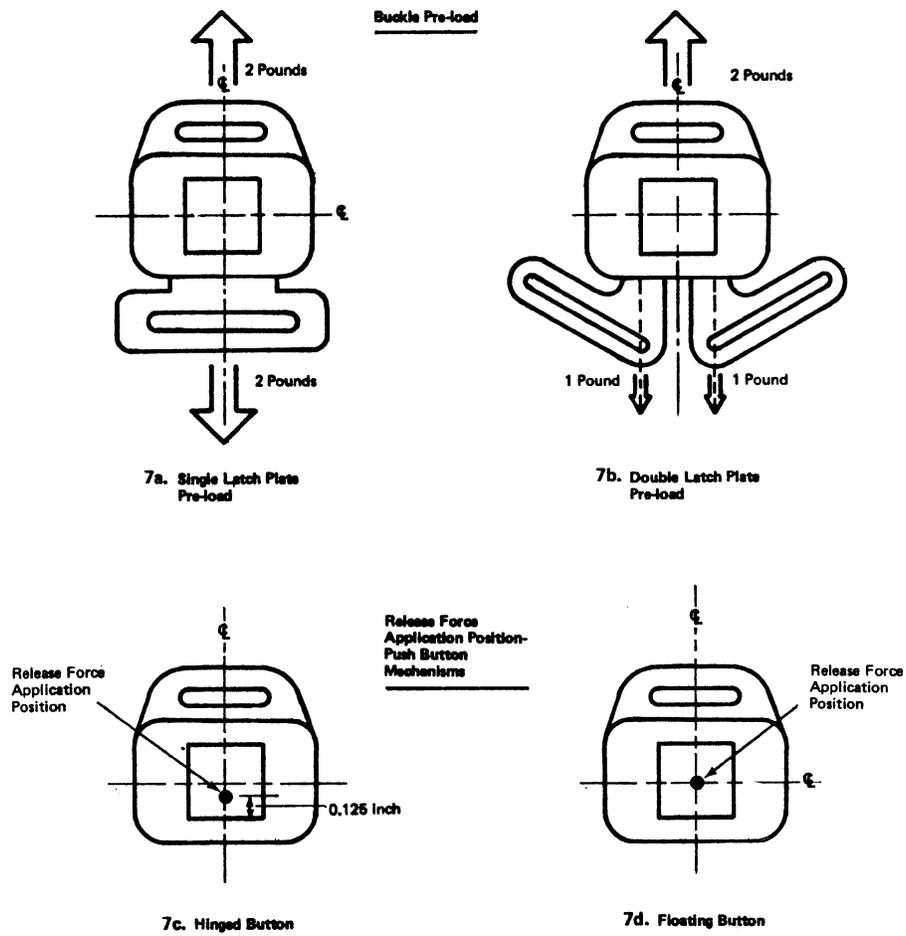
Figure 7. Pre-impact Buckle Release Force Test Set-up
